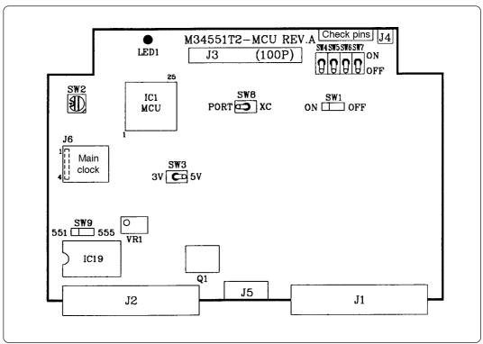
Figure 4.2 Positions of switches
